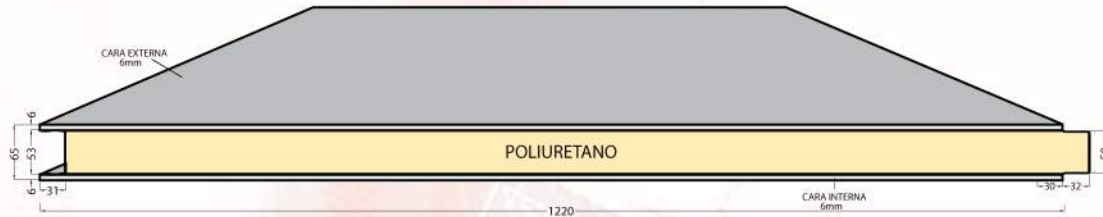
DETALLE PANEL METWALL 6+6
