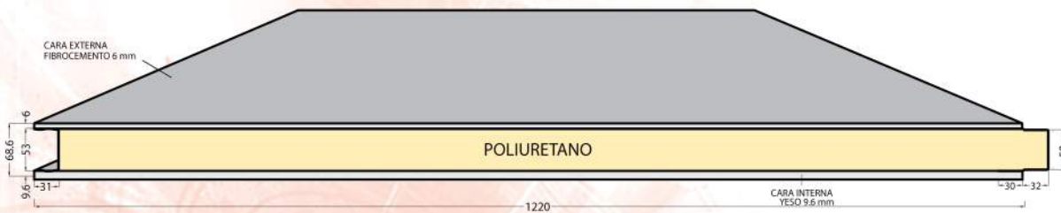
DETALLE PANEL METWALL CEMENTO / YESO 6+9.6
