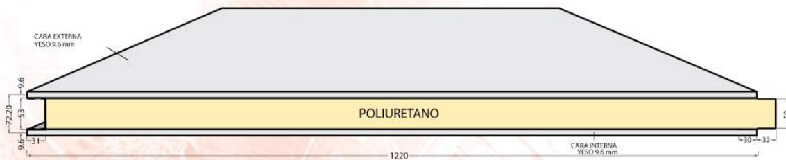
DETALLE PANEL METWALL YESO / YESO 9.6+9.6
